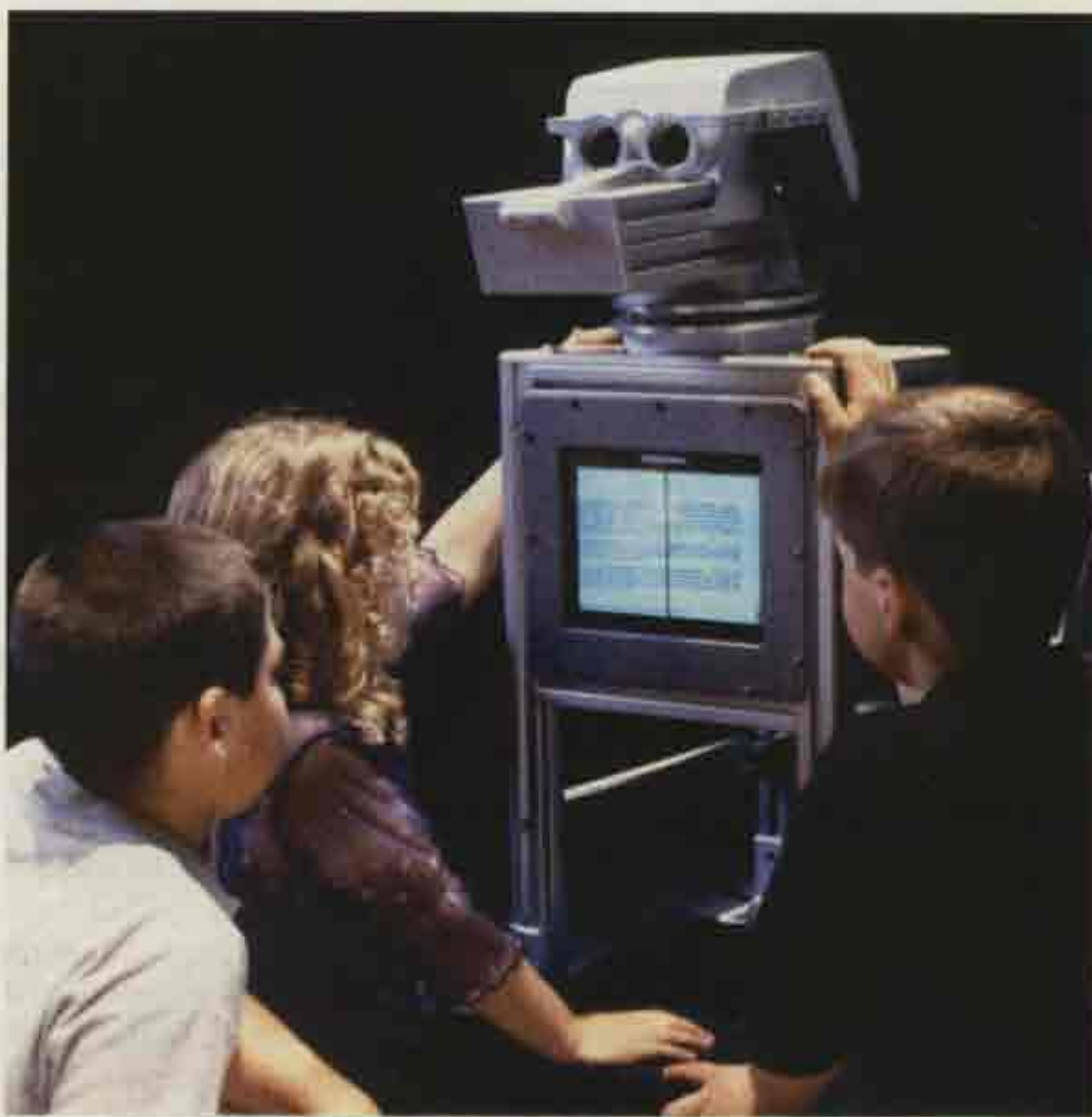
Figure 5. The Reading Eye Dog uses optical character recognition software and a text-to-voice synthesizer to read out loud to visitors.
