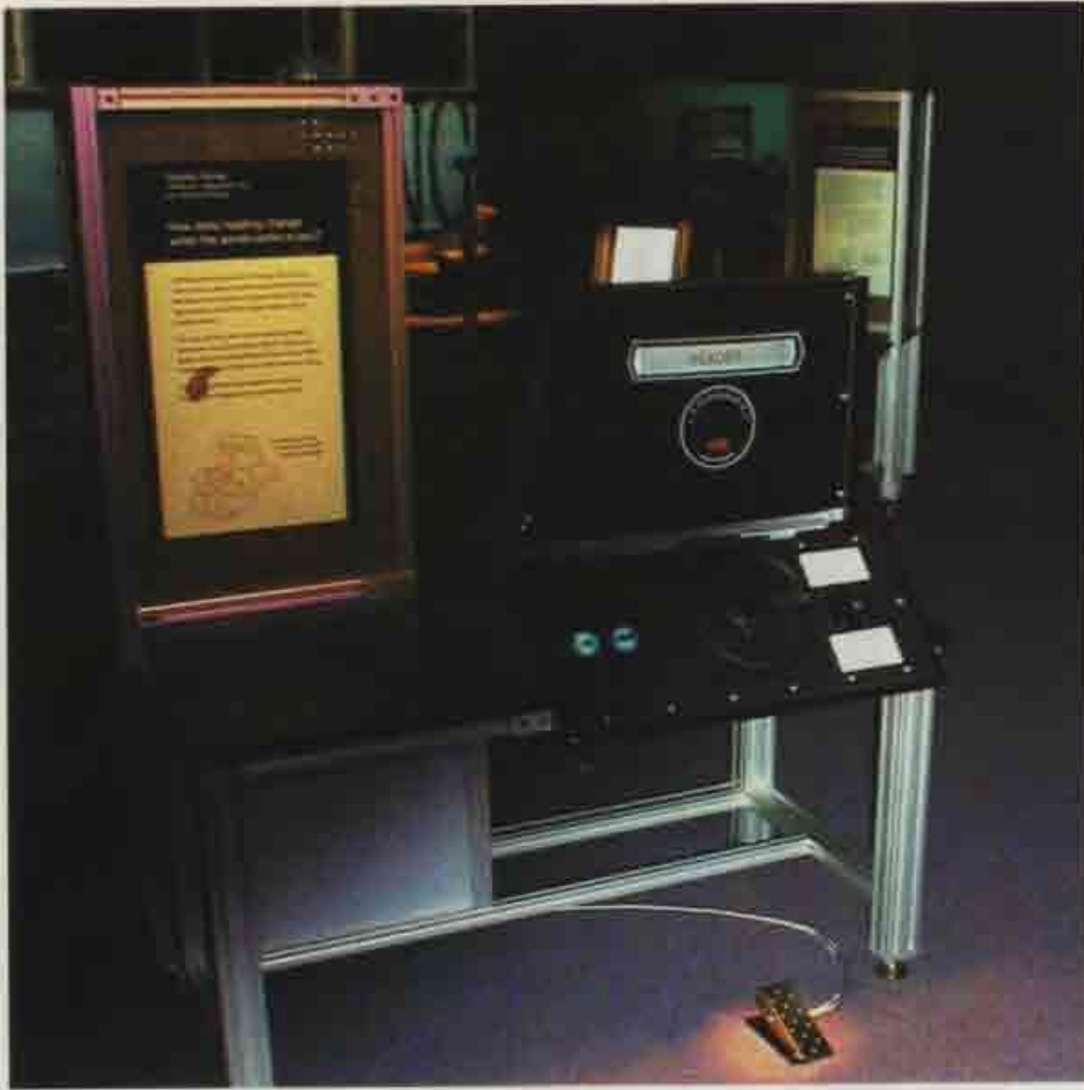
Figure 3. The Speeder Reader combines rapid serial visual presentation with a game-like racing interface to tell the story of a young girl's spaceship ride. A bright pool of tightly focused light draws attention to the speed pedal, which controls how fast words flash on the screen.
